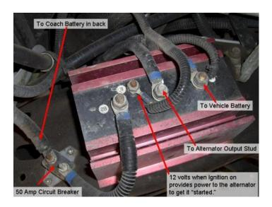
On a Chevy 190V 2002, the isolator located on a frame member under the front of the vehicle on the passenger side. I believe in most cases they are located near the engine.
