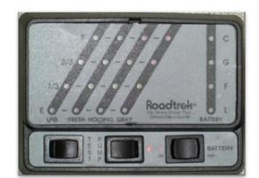
condition lights display the current battery voltage. This may or may not be representative of the battery condition. The "C" light will be on if the voltage is above about 12.7 volts, the "G" light comes on at about 12 volts, the "F" light comes on at about 11.3 volts. The "L" light will come on with less than 5 volts. This means the battery has some charge, but does not tell you much more.
